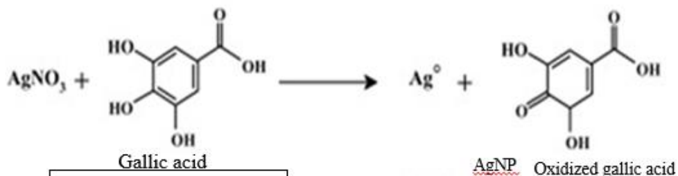
Figure 2. Reduction reaction equation of silver ions by gallic acid
